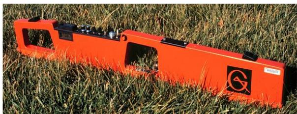
Figura 3. Sensor IM (EM38 – Geonics)
